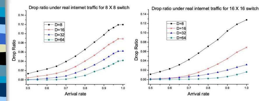
Packet drop ratio vs. *D* under Internet traffic. (a)  $8 \times 8$  switch; (b)  $16 \times 16$  switch.
