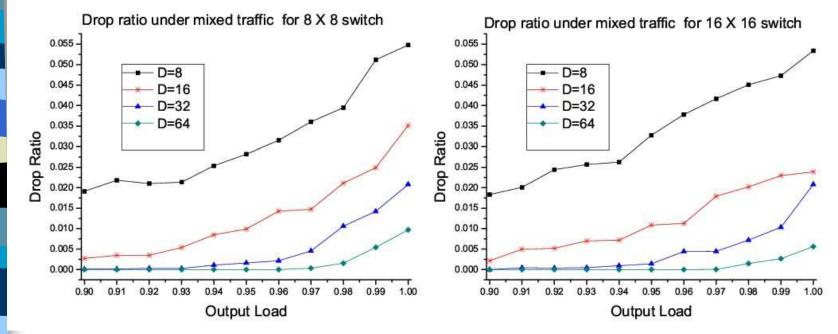
Packet drop ratio vs. *D* under mixed traffic. (a)  $8 \times 8$  switch; (b)  $16 \times 16$  switch.
