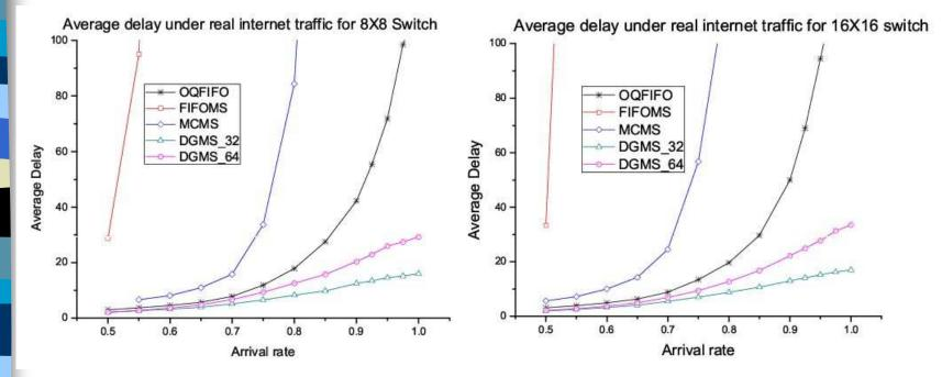
The average delay vs. arrival rate under Internet traffic. (a)  $8 \times 8$  switch; (b)  $16 \times 16$  switch.
