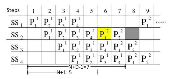
$P_j^k$ : The packet arriving from input j in the k<sub>th</sub> time slot
