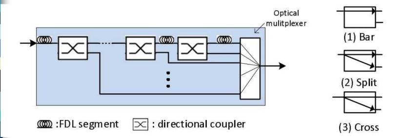
(a) The structure of M-FDL (b) 3 states of the coupler
