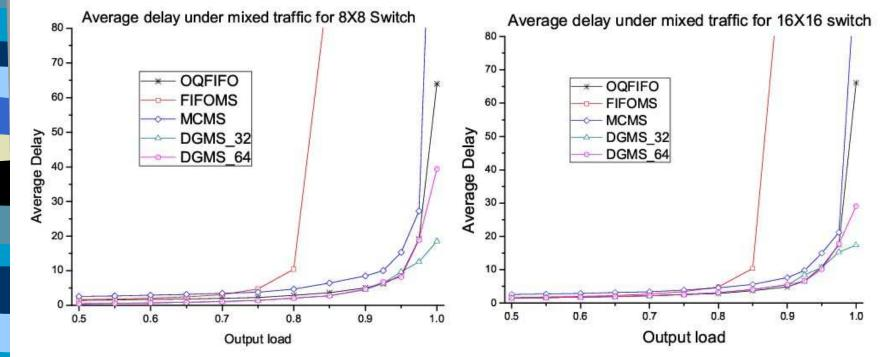
Average delay vs. output load under mixed traffic. (a)  $8 \times 8$  switch; (b) 16  $\times$  16 switch.
