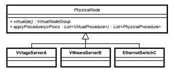
Figure 3. Class Diagram of PhysicalNode class and its Child Classes
