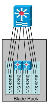
Figure 2 – Equivalent Logical Network
