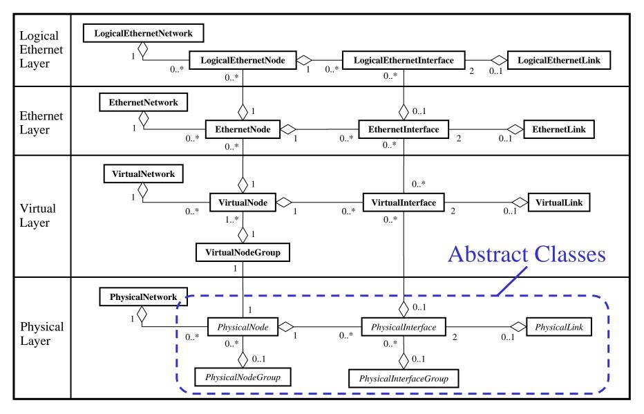
• Child classes of *PhysicalNode* class include device-specific configurations and conversion processes.
