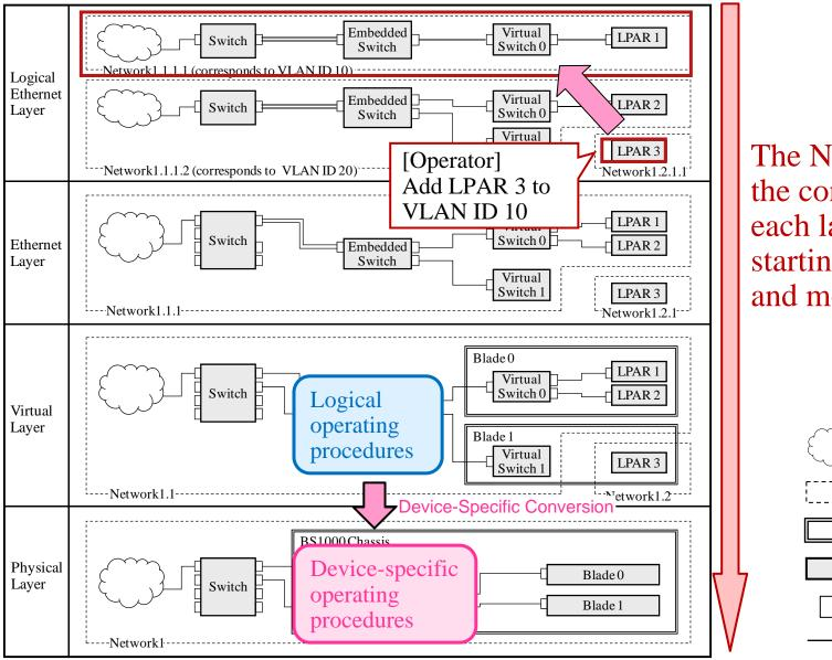
The NMS checks the connections of each layer starting from top and moving down
