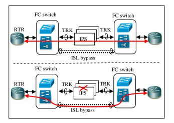
Figure 5: Bypass a critical failure
