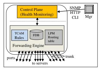
Figure 1: Flow Control switch functional view
