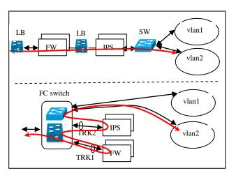
Figure 4: Packet steering with multiple inline services
